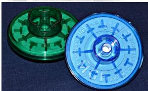
SAM bacterial and hydrophobic filters are sealed disposable air filter capsules moulded in high impact polystyrene encapsulating a bonded micro glass fibre disc.
