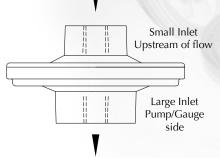
When replacing filters, particularly the hydrophobic Filter, it is important to ensure the filter is connected correctly to suit the direction of flow. The filters will only operate efficiently in one direction and the diagram opposite indicates the correct orientation when installed in-line in the pipework. However when fitted directly to the mount on a SAM unit, the base of the filter is now moulded with a 'bayonet' type fitting to ensure it can only be connected the correct way around.
